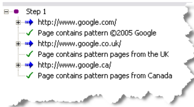
Figure D: PROGNOSIS checks for text in the HTML source to identify a web page
