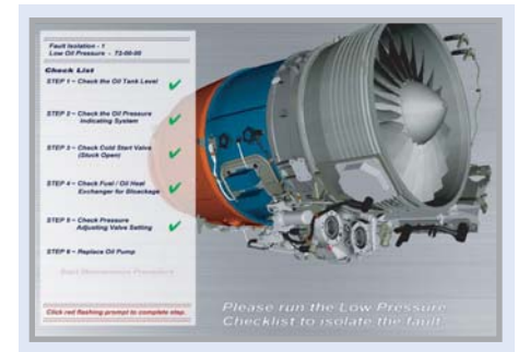
Pratt & Whitney used Right Hemisphere's Deep Creator and Deep Server to develop a real-time, interactive diagnostic system for troubleshooting aircraft engines.
